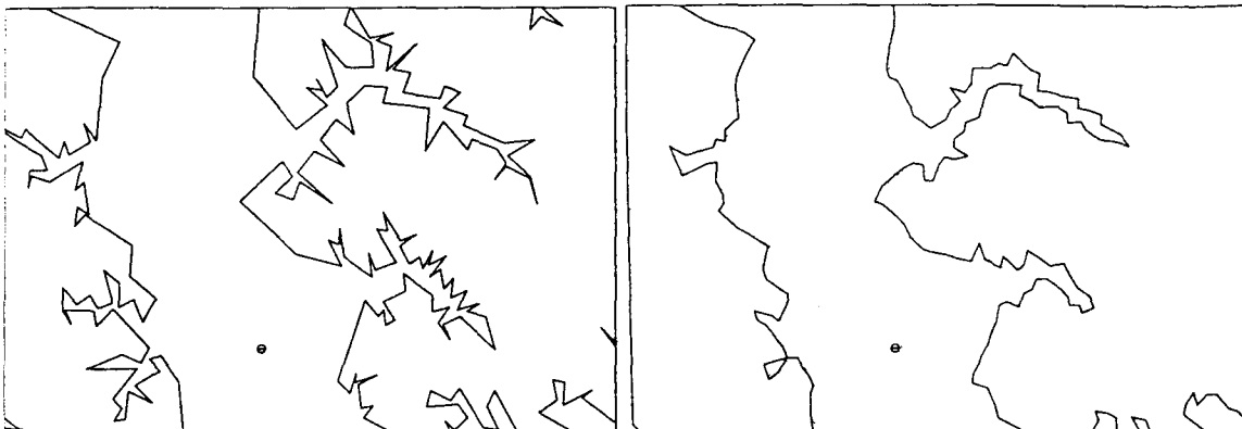
FIGURE 19. North Carolina coastline plotted at 150,000 scale: a. Douglas algorithm – 200 meter tolerance; b. WHIRLPOOL algorithm – 200 meter tolerance.
