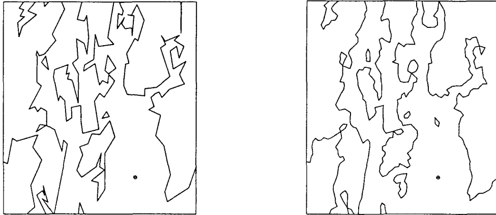
FIGURE 22. Maine coastline plotted at 125,000 scale: a. Douglas algorithm – 150 meter tolerance; b. WHIRLPOOL algorithm – 150 meter tolerance.
