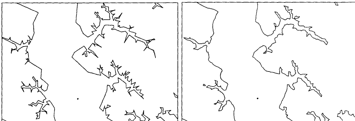
FIGURE 17. North Carolina coastline plotted at 150,000 scale: a. Douglas algorithm – 100 meter tolerance; b. WHIRLPOOL algorithm – 100 meter tolerance.
