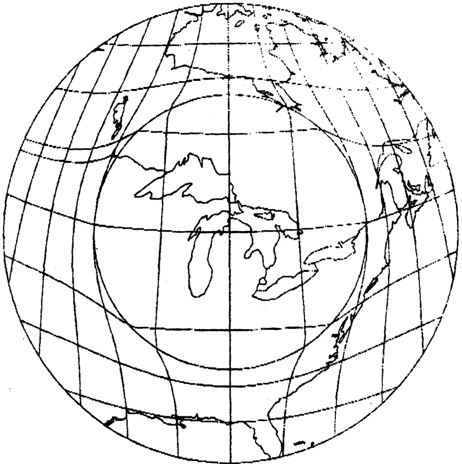
Figure 3. "Magnifying Glass" Azimuthal Equal Area projection centered at 45° N, 85° W with the inner circle at 1" radius, the outer circle at 2" radius, and the area scale factor k_a between the inner and outer circles set at 0.25.
