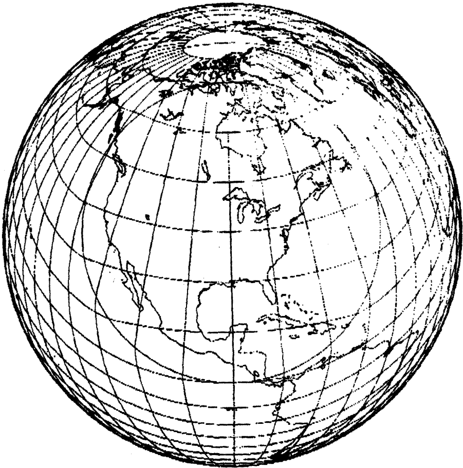
Figure 5. "Magnifying-Glass" Tapered Azimuthal Equidistant projection with the same parameters as Figure 1, except that the ratio of radii of inner to outer circles is 0.65.
