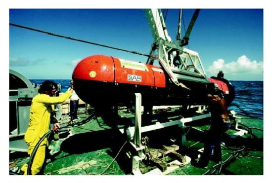
The crew of *Le Suroit* prepare to launch deep-sea sonar in 1985 during a search for the wreck of the *Titanic*. Sonar (sound navigation and ranging) uses sound to locate and identify targets, whether shipwrecks, submarines, or schools of fish.
