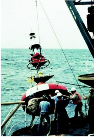
Instruments that measure physical and chemical aspects of the oceans and atmosphere can mounted on or suspended from a buoy. Together with shipboard and satellite data, the global network of measuring sites provides further understanding of the ocean-atmosphere system and its influence on global climate and biological productivity.
