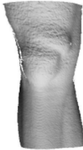
Fig. 3. The right knee. Beneath the knee is Plaster, above is Parian Marble. The contrast in noise levels is quite marked
