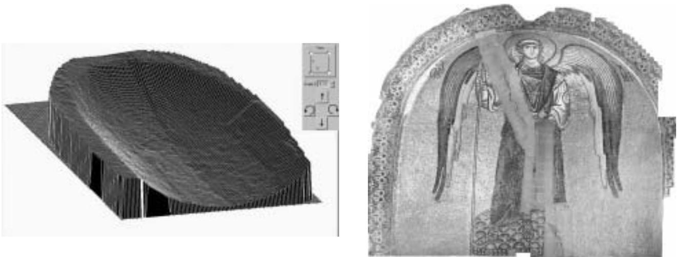
Figure 5. Test field 1: (a) 3D axonometric view of the DSM grid and (b) Orthophoto-mosaic
