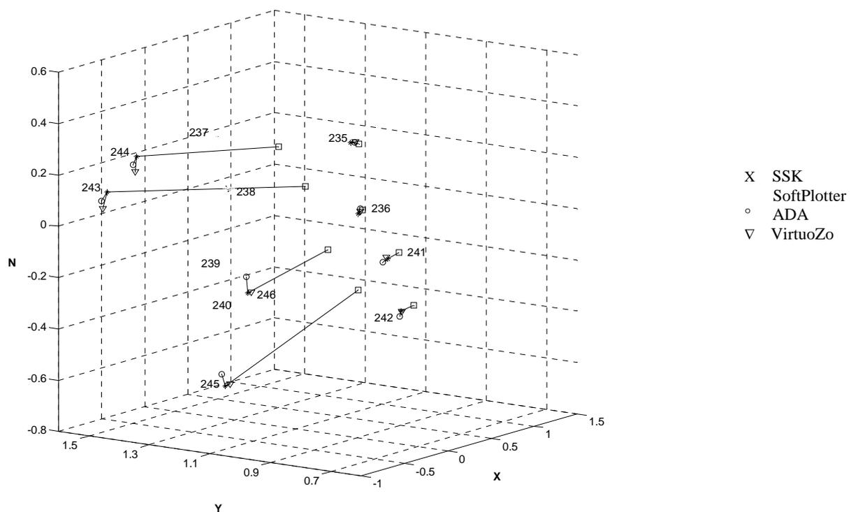
Figure 4. Test field 2 - Deviations of the camera station coordinates
