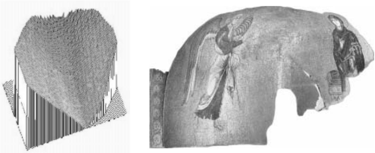
Figure 6. Test field 2: (a) 3D axonometric view of the DSM grid and (b) Orthophoto-mosaic
