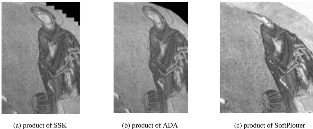
Figure 10. Visual comparison of orthophotos – Detail of test field 2
